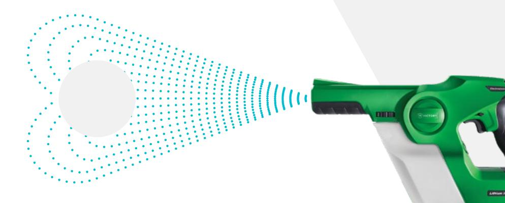
Electrostatic-sprayed particles will have an attraction up to 75 times that of gravity and will seek out items to land on versus "floating" in the air. Once the like-charged particles land upon a surface, they repel each other like magnets – spreading out evenly across the sprayed surface and providing excellent solution coverage.
